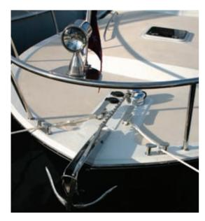
**Anchoring** The optional anchoring system features a Muir windlass with selflaunching, polished Lewmar claw anchor and 250' of bright stainless chain and ½" rode. Anchor up/down controls are at the helm and on deck.
