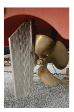
**Single Prop** A prop mounted as close as possible to a large rudder provides excellent control when you need it most. *BOATING Magazine (June '03)*
