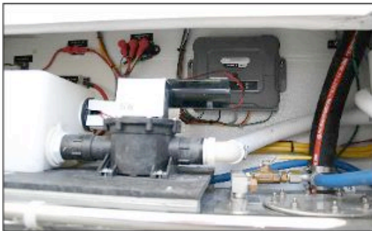
STARBOARD TANK showing fuel shut-off, VacuFlush Tank & Pump and Raymarine Autopilot Interface Box
