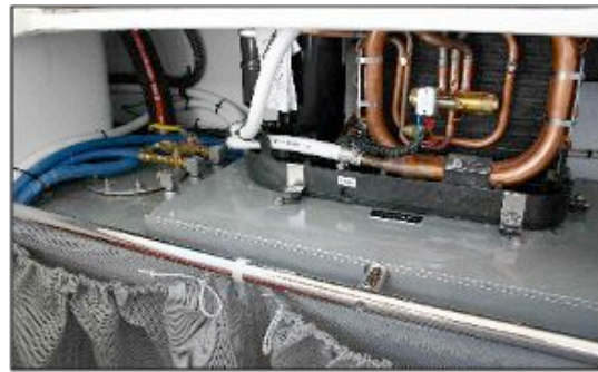
PORT TANK showing fuel shut-off for port engine as well as AC Compressor.
