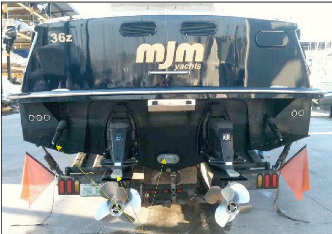
5 Zincs are seen in this photo of Volvo Drives: Trim Tab (2), Drive (2) and Transom Zinc (1) . The Yanmar Drives have zincs on the lifter arms as well as under the Drives.
